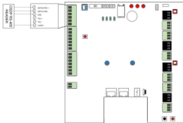
Wire Doors for OSDP Readers using RS-485
